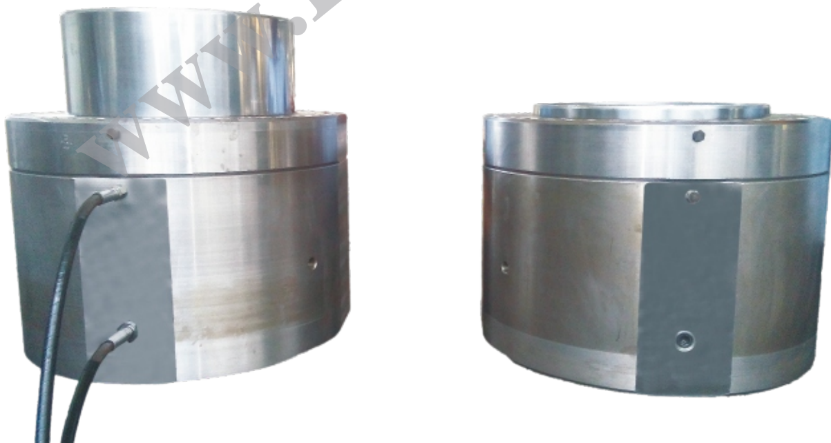
2. Typical View of a Roll Force Cylinders Bore \phi 800mm x Piston Rod \phi 750mm x Stroke 272.5mm under cyclical operation test.
